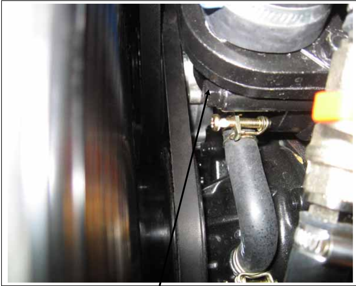
The end of the stiffener bracket with the slot bolts on this point using the \frac{3}{4} " spacer and the long M8 bolt.
